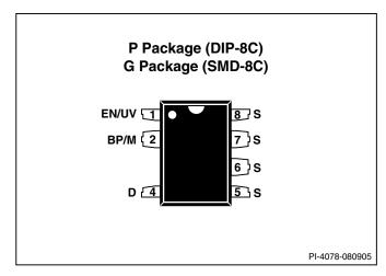
Figure 3. Pin Configuration.
