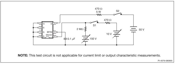
Figure 16. General Test Circuit.
