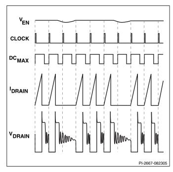
Figure 7. Operation at Moderately Heavy Loading.
