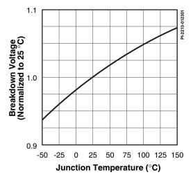
Figure 20. Breakdown vs. Temperature.
