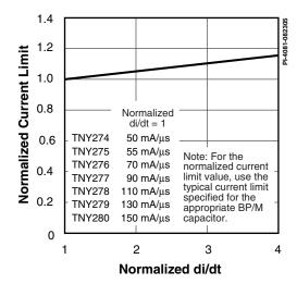
Figure 23. Current Limit vs. di/dt.
