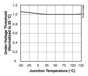
Figure 27. Undervoltage Threshold vs. Temperature.
