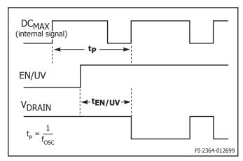
Figure 18. Output Enable Timing.
