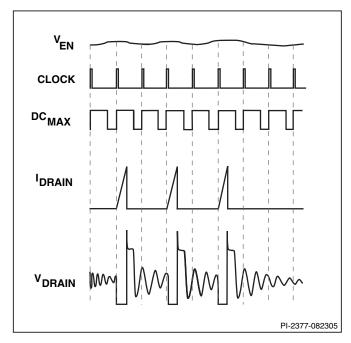
Figure 8. Operation at Medium Loading.
