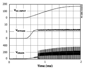
Figure 11. Power Up Without Optional External UV Resistor Connected to FN/LV Pin.
