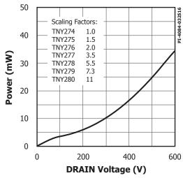
Figure 26. Drain Capacitance Power.
