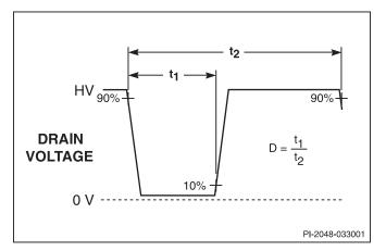
Figure 17. Duty Cycle Measurement.
