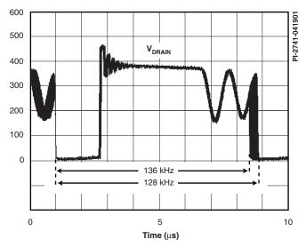
Figure 4. Frequency Jitter.
