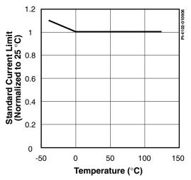
Figure 22. Standard Current Limit vs. Temperature.
