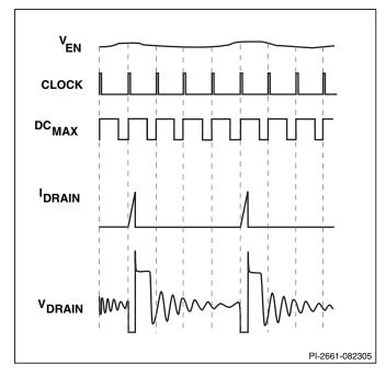
Figure 9. Operation at Very Light Load.
