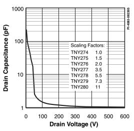
Figure 25.  $C_{\rm OSS}$  vs. Drain Voltage.
