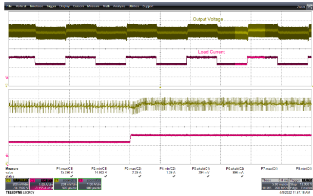
Figure 59 – Transient Response. 265 VAC, 15 V, 1.5 – 2.25 A Load Step. V_{MIN} : 14.903 V, V_{MAX} : 15.29 V. Upper: V_{OUT} , 0.2 V / div., 5 ms / div. Lower: I_{LOAD} , 1 A / div. Zoom: 0.5 ms / div.
