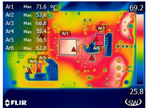
Figure 31 – Bottom Thermal Image. Ar1: InnoSwitch4-Pro, U2 = 71.6 °C. Ar2: Bus Switch, Q3 = 53.6 °C. Ar3: Clamp Zero IC = 60.8 °C. Ar4: Sec. Snubber Diode = 55.4 °C. Ar5: Sec. Schottky Diode = 56.5 °C. Ar6: BJT, Q1 = 62.8 °C.
