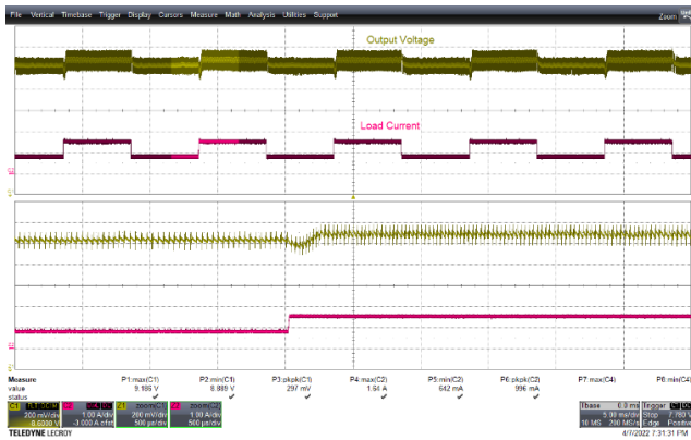
Figure 48 – Transient Response. 90 VAC, 9.0 V, 0.75 – 1.5 A Load Step. V_{MIN} : 8.889 V, V_{MAX} : 9.186 V. Upper: V_{OUT} , 0.2 V / div., 5 ms / div. Lower: I_{LOAD} , 1 A / div. Zoom: 0.5 ms / div.
