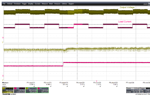
Figure 44 – Transient Response. 90 VAC, 5.0 V, 2.25 – 3 A Load Step. V_{MIN} : 4.996 V, V_{MAX} : 5.296 V. Upper: V_{OUT} , 0.2 V / div., 5 ms / div. Lower: I_{LOAD} , 1 A / div. Zoom: 0.5 ms / div.
