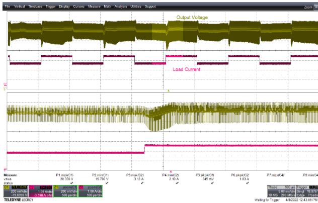
Figure 68 – Transient Response. 90 VAC, 20 V, 2.25 – 3 A Load Step. V_{MIN} : 19.706V, V_{MAX} : 20.33 V. Upper: V_{OUT} , 0.2 V / div., 5 ms / div. Lower: I_{LOAD} , 1 A / div. Zoom: 0.5 ms / div.
