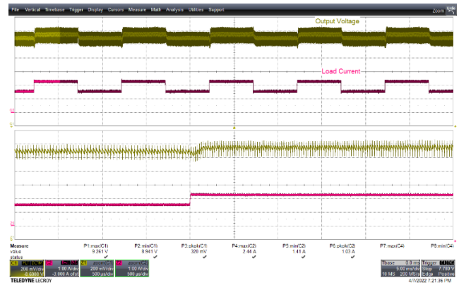
Figure 51 – Transient Response. 265 VAC, 9.0 V, 1.5 – 2.25 A Load Step. V_{MIN} : 8.941 V, V_{MAX} : 9.261 V. Upper: V_{OUT} , 0.2 V / div., 5 ms / div. Lower: I_{LOAD} , 1 A / div. Zoom: 0.5 ms / div.
