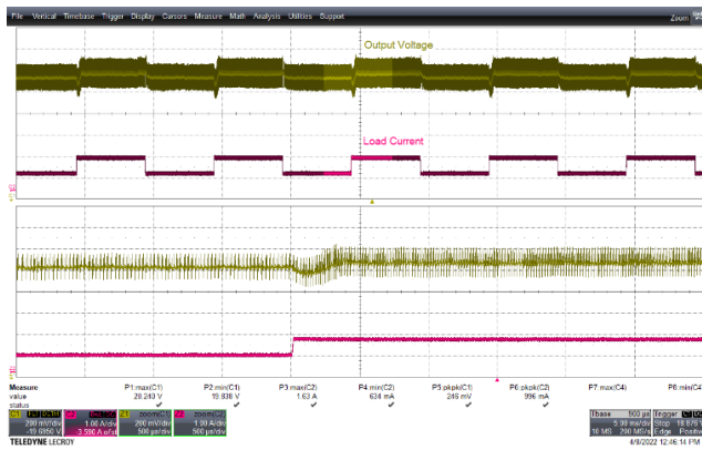
Figure 64 – Transient Response. 90 VAC, 20 V, 0.75 – 1.5 A Load Step. V_{MIN} : 19.838 V, V_{MAX} : 20.24 V. Upper: V_{OUT} , 0.2 V / div., 5 ms / div. Lower: I_{LOAD} , 1 A / div. Zoom: 0.5 ms / div.
