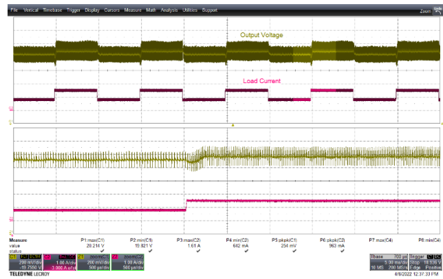
Figure 65 – Transient Response. 265 VAC, 20 V, 0.75 – 1.5 A Load Step. V_{MIN} : 19.821 V, V_{MAX} : 20.214 V. Upper: V_{OUT} , 0.2 V / div., 5 ms / div. Lower: I_{LOAD} , 1 A / div. Zoom: 0.5 ms / div.
