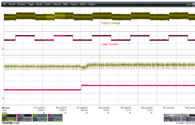
Figure 50 – Transient Response. 90 VAC, 9.0 V, 1.5 – 2.25 A Load Step. V_{MIN} : 8.934 V, V_{MAX} : 9.254 V. Upper: V_{OUT} , 0.2 V / div., 5 ms / div. Lower: I_{LOAD} , 1 A / div. Zoom: 0.5 ms / div.
