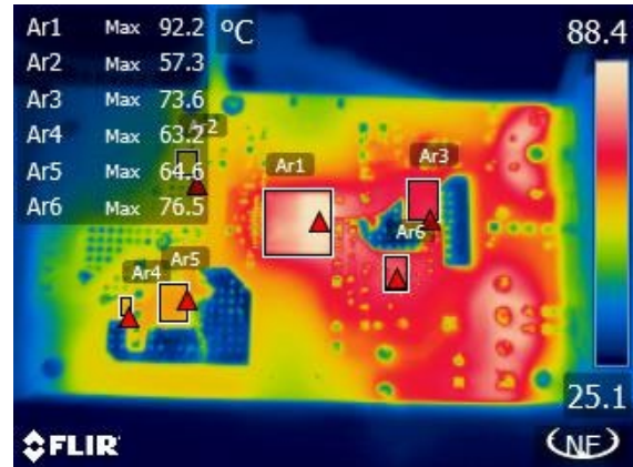
Figure 35 – Bottom Thermal Image. Ar1: InnoSwitch4-Pro, U2 = 92.2 °C. Ar2: Bus Switch, Q3 = 57.3 °C. Ar3: Clamp Zero IC = 73.6 °C. Ar4: Sec. Snubber Diode = 63.2 °C. Ar5: Sec. Schottky Diode = 64.6 °C. Ar6: BJT, Q1 = 76.5 °C.
