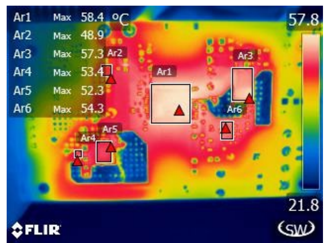
Figure 33 – Bottom Thermal Image. Ar1: InnoSwitch4-Pro, U2 = 58.4 °C. Ar2: Bus Switch, Q3 = 48.9 °C. Ar3: Clamp Zero IC = 57.3 °C. Ar4: Sec. Snubber Diode = 53.4 °C. Ar5: Sec. Schottky Diode = 52.3 °C. Ar6: BJT, Q1 = 54.3 °C.
