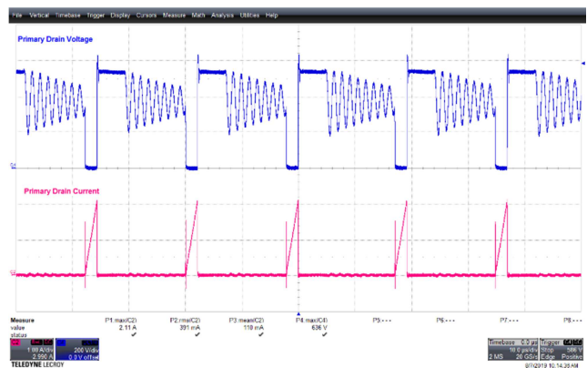
Figure 130 – 265 VAC 50 Hz, V_{USB-C} = 20\text{ V} Full Load. Upper: V_{DRAIN} , 1 A / div. Lower: I_{DRAIN} , 200 V / div., 10 \mu\text{s} / div. I_{DS} = 2.11\text{ A} , V_{DS} = 636\text{ V} .
