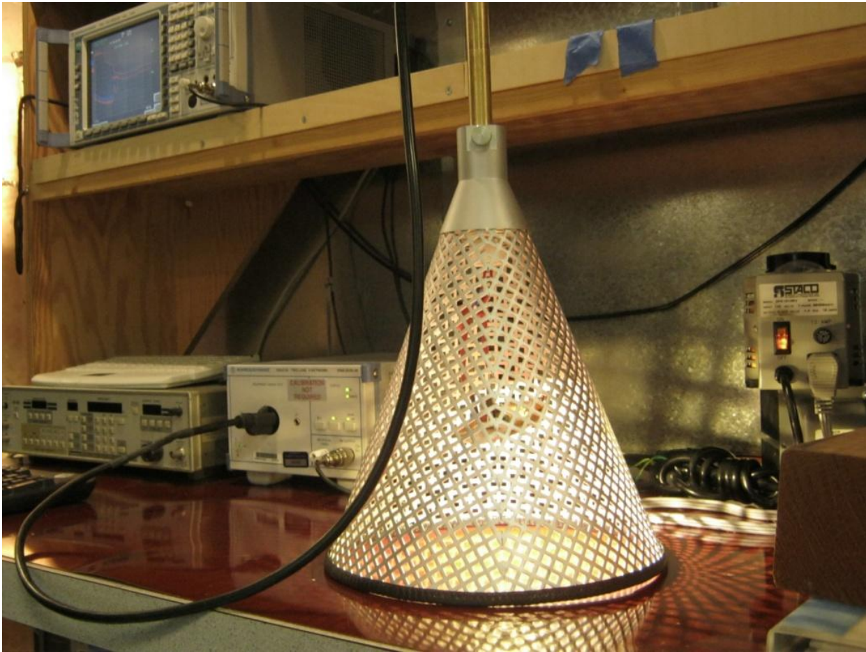
Figure 57 – EMI Test Set-up with the Unit and LED Load Placed Inside a Conical Metal Housing as Described in CISPR 15 / IEC: 2005 Standard.
