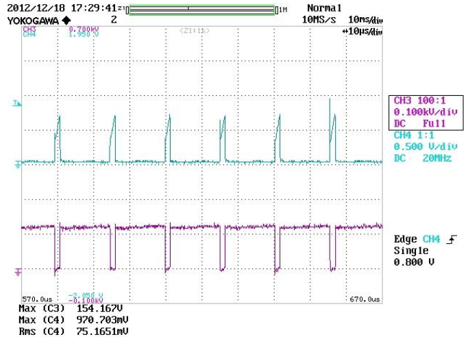
Figure 44 – 90 VAC, 60 Hz Start-up. Upper: I_{DRAIN} , 500 mA / div. Lower: V_{DRAIN} , 100 V, 10 \mu s / div.
