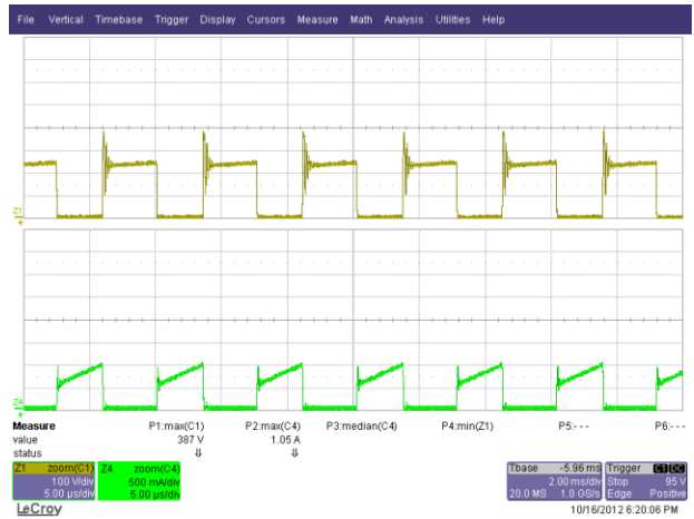
Figure 35 – 90 VAC, 60 Hz. Upper: V_{DRAIN} , 100 V / div. Lower: I_{DRAIN} , 500 mA, 5 \mu s / div.
