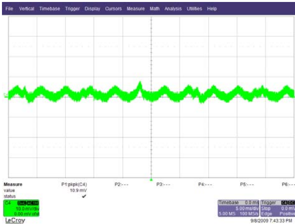
Figure 29 – 5 V Output Ripple [10.9 mV P-P ], 265 VAC, 50 Hz, Full Load. 10 mV, 5 ms / div.
