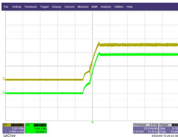
Figure 17 – Start-up Profile, 265 VAC. Upper: V_5 , 2 V / div. Lower: V_{14.5} , 5 V, 20 ms / div.
