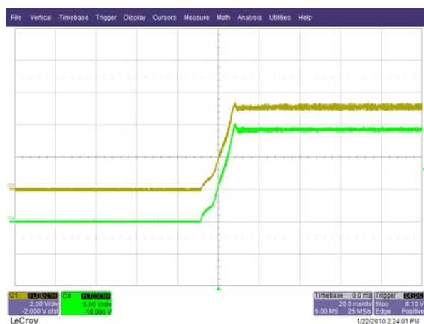
Figure 16 – Start-up Profile, 90 VAC. Upper: V_5 , 2 V / div. Lower: V_{14.5} , 5 V, 20 ms / div.
