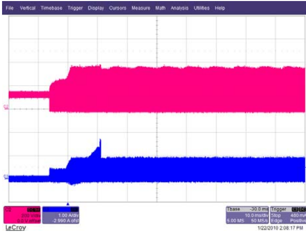
Figure 18 – 90 VAC Input and Full Load. Upper: V_{DRAIN} , 200 V / div. Lower: I_{DRAIN} , 0.5 A ,10 ms / div.
