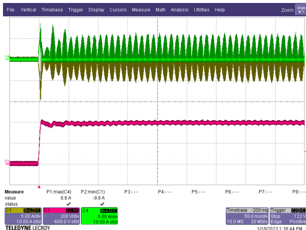
Figure 47 – 264 VAC, 100% Load. Grn: T4 Inductor Current, 10 A / div. Yel: T1 Inductor Current, 10 A / div. Red: V OUT , 200 V, 50 ms/ div.
