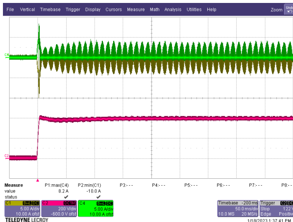
Figure 48 – 264 VAC, 50% Load. Grn: T4 Inductor Current, 10 A / div. Yel: T1 Inductor Current, 10 A / div. Red: V OUT , 200 V, 50 ms/ div.
