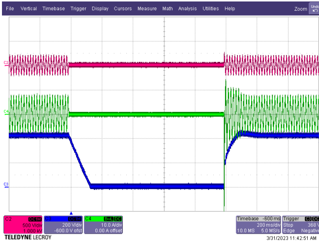
Figure 64 – Line Dropout 115 VAC, 1000 ms. Upper: V_{IN} , 200 V / div. Middle: I_{IN} , 10 A / div. Lower: V_{OUT} , 200 V / div., 200 ms / div.
