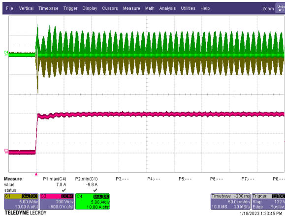
Figure 44 – 230 VAC, 100% Load. Grn: T4 Inductor Current, 10 A / div. Yel: T1 Inductor Current, 10 A / div. Red: V OUT , 200 V, 50 ms/ div.
