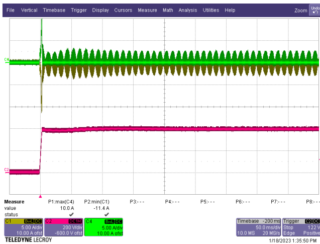
Figure 46 – 230 VAC, 25% Load. Grn: T4 Inductor Current, 10 A / div. Yel: T1 Inductor Current, 10 A / div. Red: V OUT , 200 V, 50 ms/ div.
