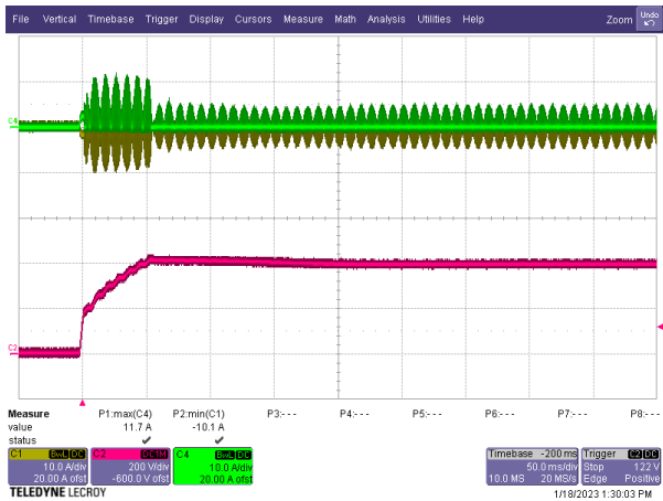
Figure 43 – 115 VAC, 25% Load. Grn: T4 Inductor Current, 10 A / div. Yel: T1 Inductor Current, 10 A / div. Red: V OUT , 200 V, 50 ms/ div.
