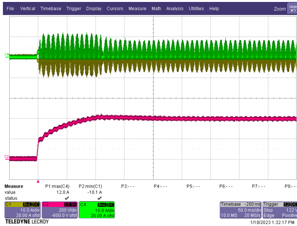
Figure 41 – 115 VAC, 100% Load. Grn: T4 Inductor Current, 10 A / div. Yel: T1 Inductor Current, 10 A / div. Red: V OUT , 200 V, 50 ms/ div.
