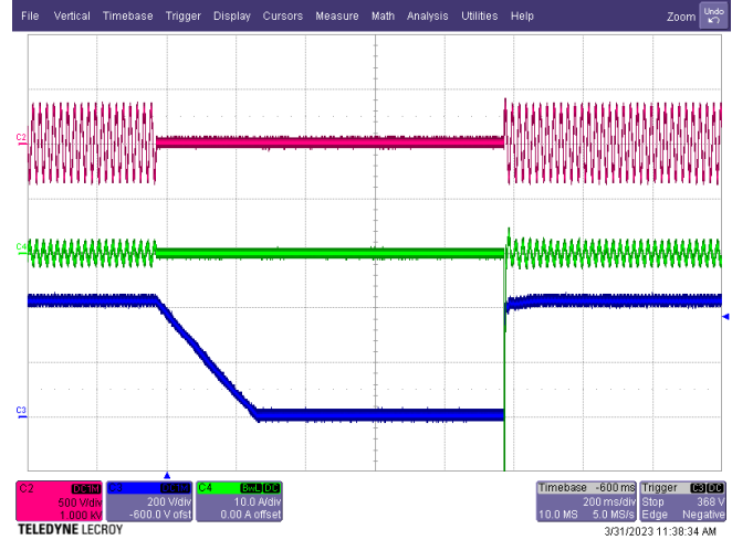
Figure 63 – Line Dropout 230 VAC, 1000 ms. Upper: V_{IN} , 500 V / div. Middle: I_{IN} , 10 A / div. Lower: V_{OUT} , 200 V / div., 200 ms / div.
