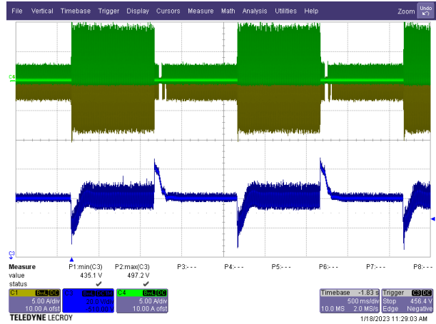
Figure 51 – Transient Response, 90 VAC, 10-100-10% Load Step. Grn: T1 Inductor Current, 5 A / div. Yel: T4 Inductor Current, 5 A / div. Blu: V_{OUT} (DC Coupled), 20 V, 500 ms / div.
