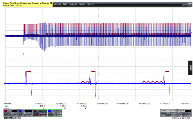
Figure 50 – Primary Clamp Drain Voltage and Current. 265 VAC, 5 V, 3 A Load (454 V MAX ). C1: V DRAIN , 200 V / div. C2: I DRAIN , 500 mA / div. Time (Zoom): 20 μs / div.
