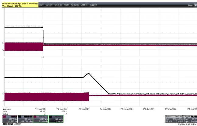
Figure 101 – Output Overvoltage Test. 90 VAC, 28 V, 5 A Load. C1: V_{DS} , 500 V / div. C4: V_{OUT} , 10 V / div. V_{OMAX} : 35 V. Time (Zoom): 7.2 ms / div.
