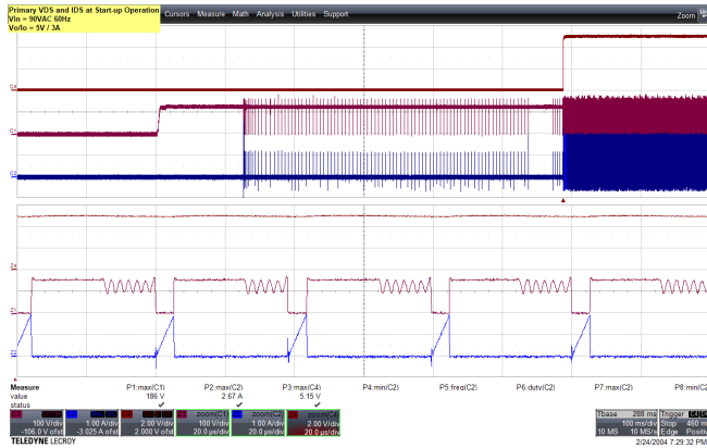
Figure 47 – InnoSwitch4-CZ Drain Voltage and Current. 90 VAC, 5 V, 3 A Load (191 V MAX ). C1: V DRAIN , 100 V / div. C2: I DRAIN , 1 A / div. Time (Zoom): 19.4 μs / div.
