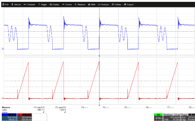
Figure 15 – Drain Voltage and Current. V_{IN} = 130 \text{ VDC} , I_{OUT} = 1.67 \text{ A} . CH1: V_{DRAIN-SOURCE} , 50 V, 10 \mu\text{s} / div. CH2: I_{DRAIN} , 200 mA, 10 \mu\text{s} / div. V_{DS(MAX)} = 280.1 \text{ V} , I_{DRAIN(MAX)} = 1.254 \text{ A} . V_{DS} derating: 37.35 %.
