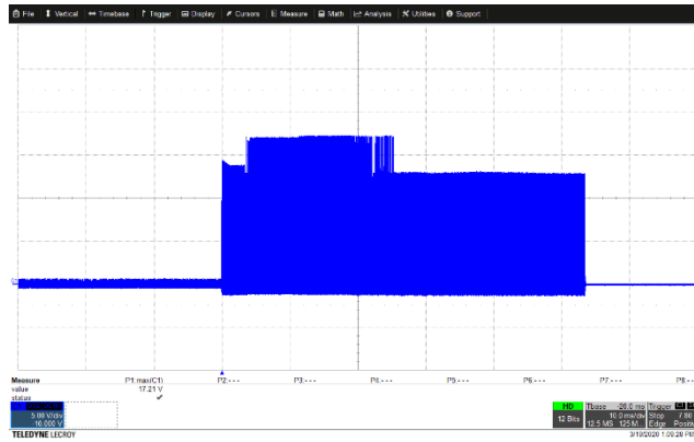
Figure 54 – FWD Pin Voltage. V_{IN} = 60 \text{ VDC} , Output Shorted. CH1: V_{FWD} , 5 V, 10 ms / div. V_{FWD(MAX)} = 17.21 \text{ V} (<150 \text{ V}) .
