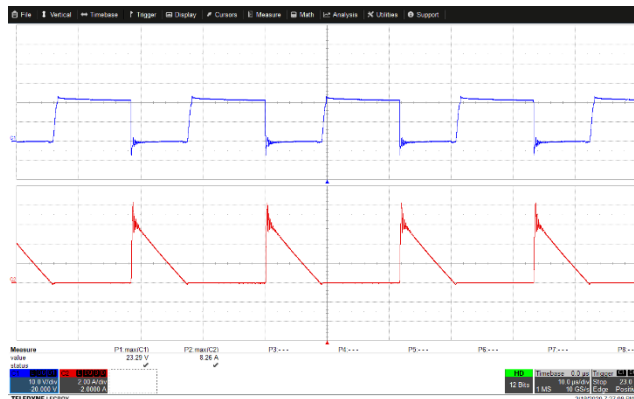
Figure 29 – Drain Voltage and Current. V_{IN} = 60 \text{ VDC} , I_{OUT} = 1.25 \text{ A} . CH1: V_{DRAIN-SOURCE} , 10 V, 10 \mu\text{s} / div. CH2: I_{DRAIN} , 2 A, 10 \mu\text{s} / div. V_{DS(MAX)} = 23.29 \text{ V} , I_{DRAIN(MAX)} = 8.26 \text{ A} . V_{DS} derating: 11.64 %.
