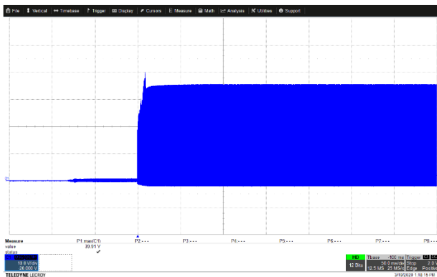
Figure 50 – FWD Pin Voltage. V_{IN} = 130 \text{ VDC} , I_{OUT} = 1.67 \text{ A} . CH1: V_{FWD} , 10 V, 50 ms / div. V_{FWD(MAX)} = 39.91 \text{ V} (<150 \text{ V}) .
