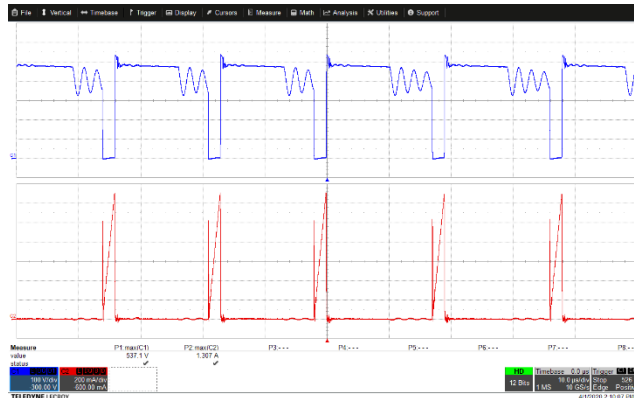
Figure 59 – Drain Voltage and Current. V_{IN} = 400 \text{ VDC} , I_{OUT} = 2.08 \text{ A} . CH1: V_{DRAIN-SOURCE} , 100 V, 10 \mu\text{s} / div. CH2: I_{DRAIN} , 200 mA, 10 \mu\text{s} / div. V_{DS(MAX)} = 537.1 \text{ V} , I_{DRAIN(MAX)} = 1.307 \text{ A} . V_{DS} derating: 71.61 %.
