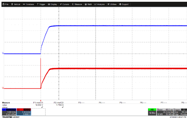
Figure 66 – Output Voltage and Current. V_{IN} = 130 VDC, Load = 6.67 \Omega . CH1: V_{OUTPUT} , 5 V, 20 ms / div. CH2: I_{OUTPUT} , 1 A, 20 ms / div.
