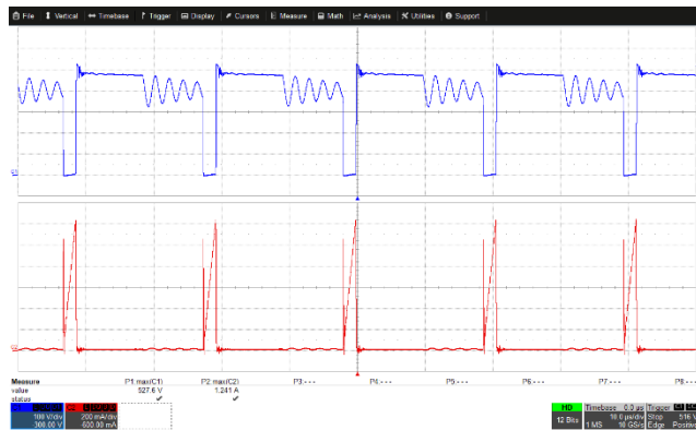
Figure 16 – Drain Voltage and Current. V_{IN} = 400 \text{ VDC} , I_{OUT} = 1.67 \text{ A} . CH1: V_{DRAIN-SOURCE} , 100 V, 10 \mu\text{s} / div. CH2: I_{DRAIN} , 200 mA, 10 \mu\text{s} / div. V_{DS(MAX)} = 527.6 \text{ V} , I_{DRAIN(MAX)} = 1.241 \text{ A} . V_{DS} derating: 70.35 %.
