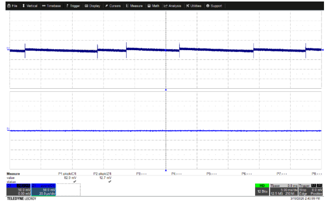
Figure 94 – Output Voltage Ripple. V_{IN} = 400 \text{ VDC} , I_{OUT} = 0 \text{ A} . CH1: V_{OUT(mVpp)} , 50 mV, 5 ms / div. Zoom: 20 \mu\text{s} / div. V_{RIPPLE(PK-PK)} = 82.9 \text{ mV}_{pp} .
