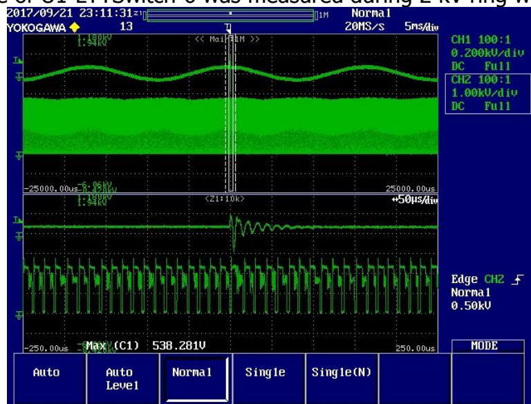
Figure 96 – (+) 2.5 kV Ring Wave Surge. 90° Phase Angle, Input: 230 VAC. V_{DRAIN} , 200 V / div., 20 ms / div. Peak V_{DRAIN} : 558.333 V.
