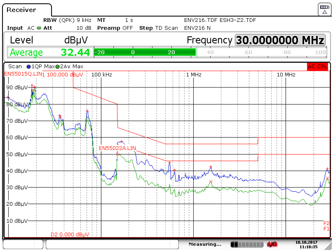
Figure 93 – Conducted EMI QP Scan at Full Load, 230 VAC 60 Hz and EN55015 B Limits.
