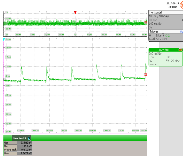
Figure 83 – 230 VAC 50 Hz, 58 mA LED Load. AC Coupling, 20 MHz Bandwidth. V_{OUT} , 200 mV / div., 100 ms / div. Ripple Voltage: 466.4 mV PK-PK .
