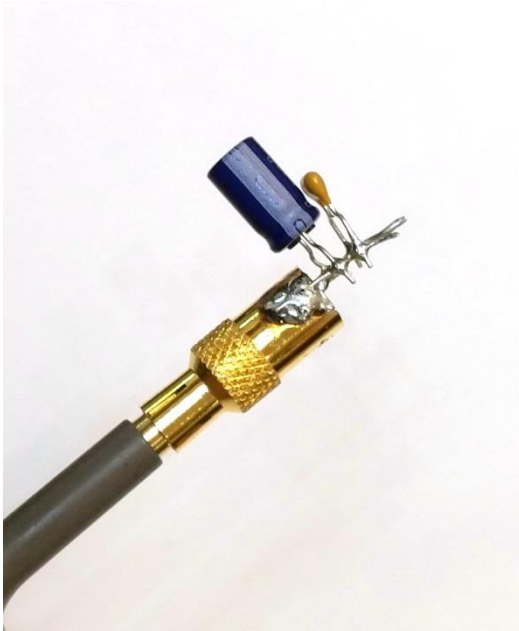
Figure 76 – Probe Set-up for Output Voltage Ripple Test.
