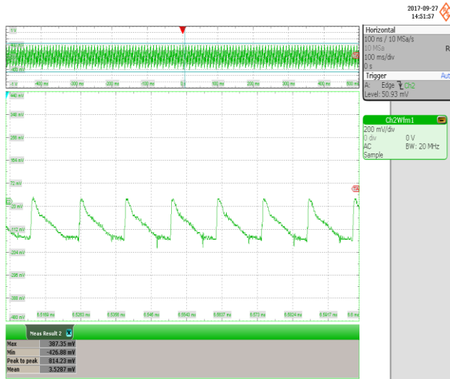
Figure 82 – 230 VAC 50 Hz, 580 mA LED Load. AC Coupling, 20 MHz Bandwidth. V_{OUT} , 200 mV / div., 100 ms / div. Ripple Voltage: 814.23 mV PK-PK .
