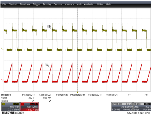
Figure 37 – Drain Voltage and Current Waveforms. 85 VAC, 9.0 V, 2 A Load, (262 V MAX ). Upper: V DRAIN , 100 V / div. Lower: I DRAIN , 500 mA / div., 20 µs / div.
