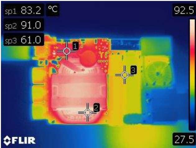
Figure 52 – Top Thermal Image. SP1: SR FETs = 83.2 °C. SP2: Bulk Capacitors = 91.0 °C. SP3: Winding PCB = 61.0 °C.
