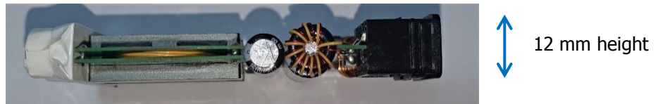
Figure 5 – Populated Circuit Board Photograph - Side.
