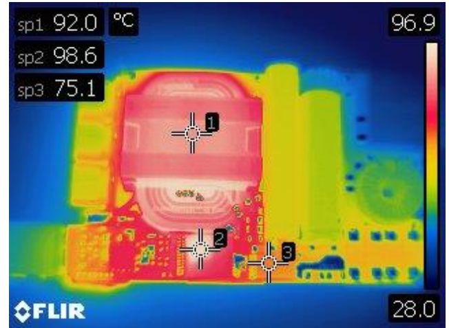
Figure 53 – Bottom Thermal Image. SP1: Transformer Core = 92.0 °C. SP2: InnoSwitch3-Pro = 98.6 °C. SP3: MinE-CAP = 75.1 °C.
