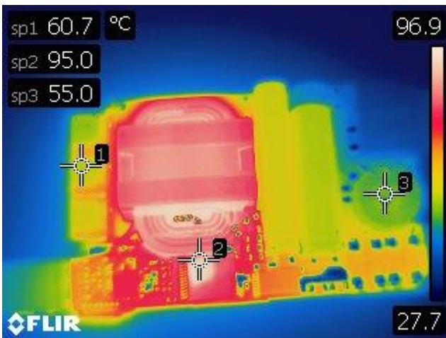
Figure 54 – Bottom Thermal Image. SP1: Output Capacitors = 60.7 °C. SP2: InnoSwitch3-Pro = 95.0 °C. SP3: CMC L2 = 75.1 °C.
