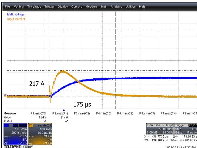
Figure 15. Inrush Current for  $V_{IN} = 115 \text{ VAC}$  and  $100 \mu\text{F}$  Input Capacitor without MinE-CAP IC Circuit.
