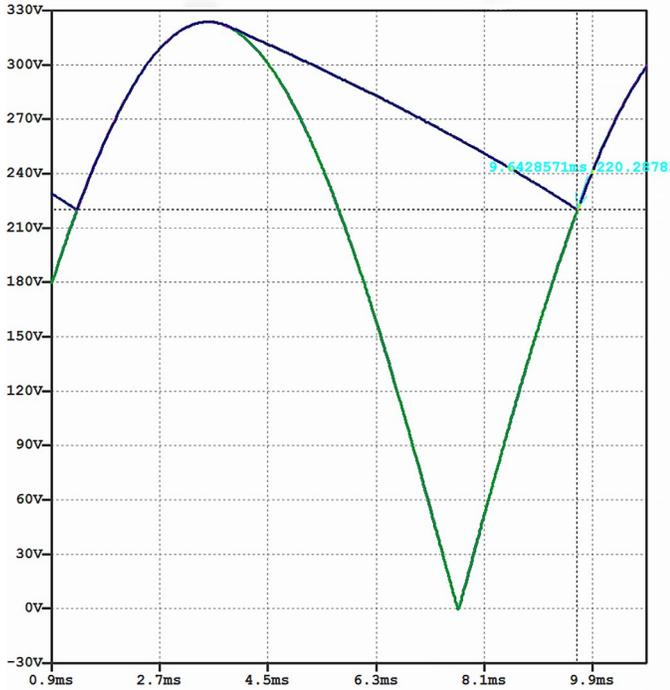
Figure 28. Circuit Simulation of Figure 9 using  $P_o = 65 \text{ W}$ ,  $\eta = 0.92$ ,  $V_{IN} = 230 \text{ VAC}$  and  $C_{BULK} = 15 \mu\text{F}$ ; Rectified Voltage (Green), Capacitor Voltage (Blue).
