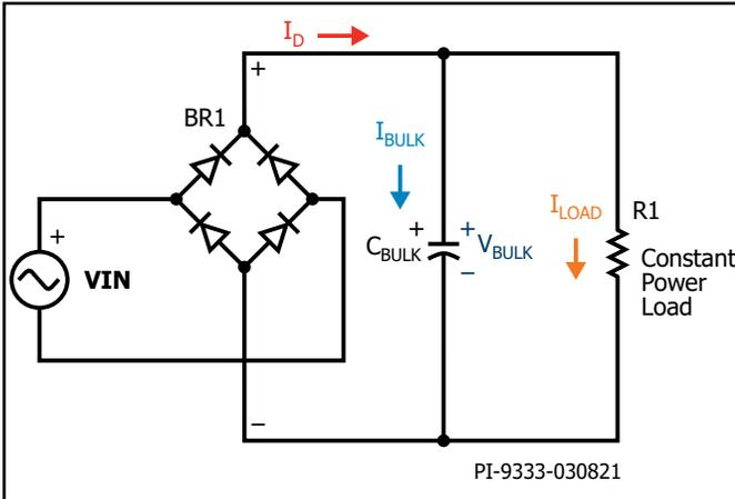
Figure 26. Basic Rectifier Circuit with Constant Power Load.
