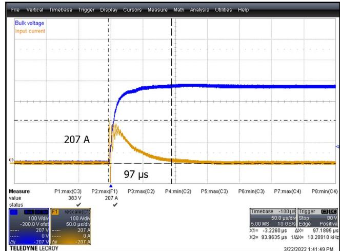
Figure 16. Inrush Current for  $V_{IN} = 265 \text{ VAC}$  and  $100 \mu\text{F}$  Input Capacitor with MinE-CAP IC Circuit.
