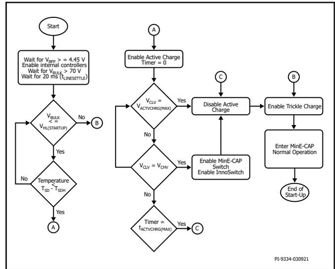
Figure 9. MinE-CAP Start-up Flowchart.
