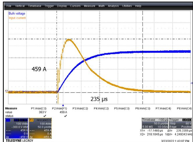
Figure 17. Inrush Current for  $V_{IN} = 265 \text{ VAC}$  and  $100 \mu\text{F}$  Input Capacitor without MinE-CAP IC Circuit.
