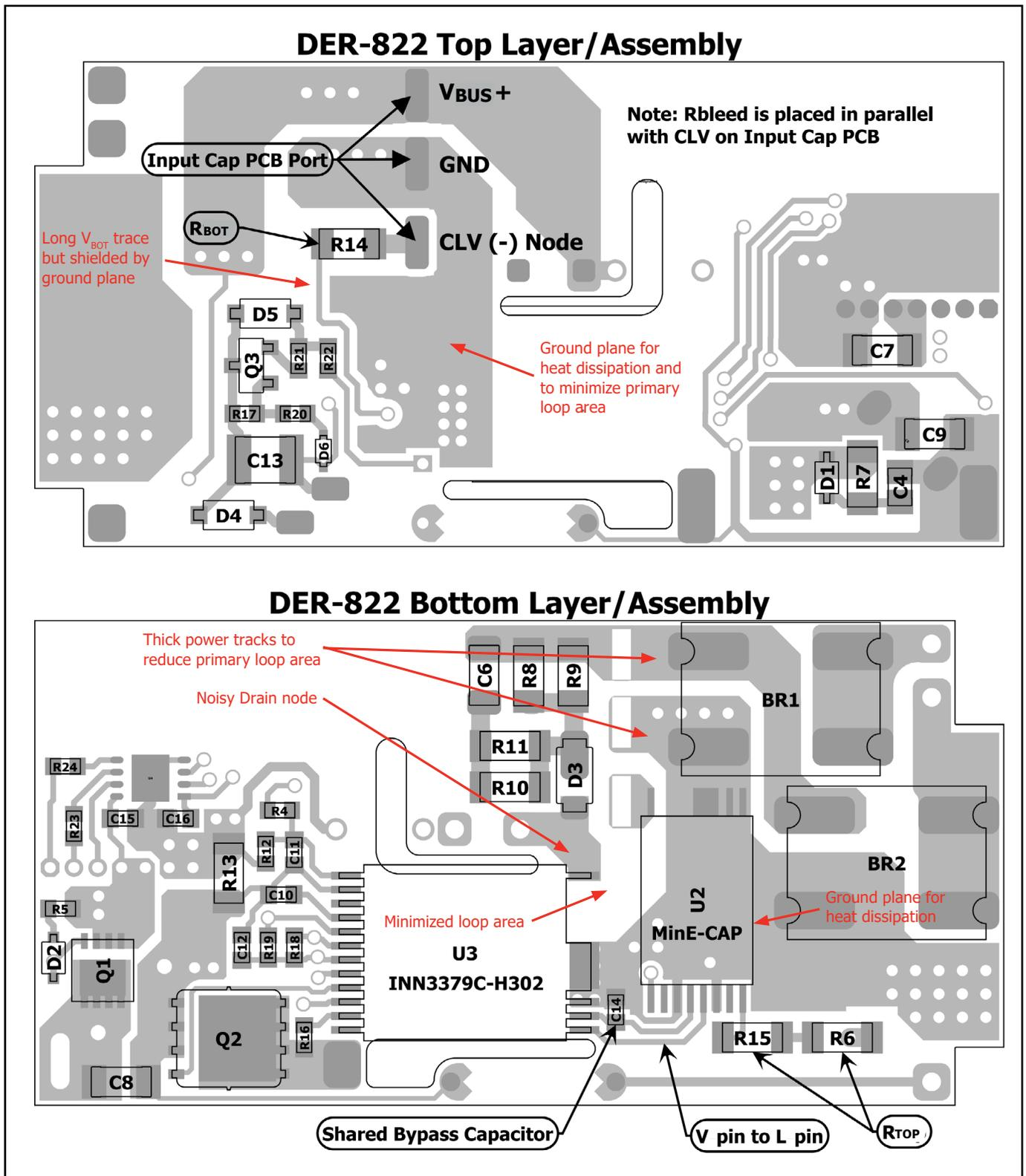
Figure 25. MinE-CAP IC Circuit Example Layout from DER-822 (60 W USB-C PD using INN3379C-H302).
