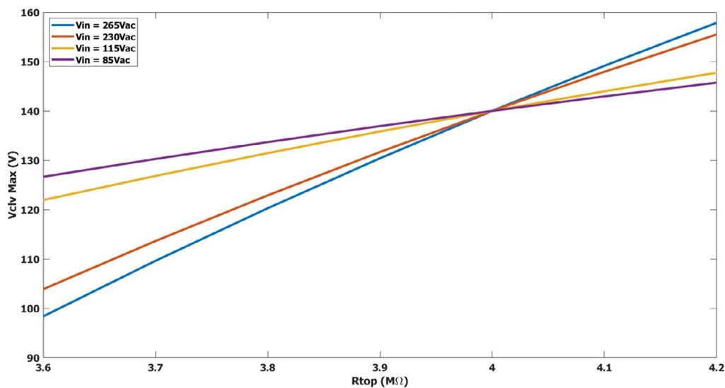
Figure 7. Maximum Voltage Across  $C_{LV}$  vs. Varying  $R_{TOP}$ ;  $R_{BOT} = 1.0\text{ M}\Omega$ .
