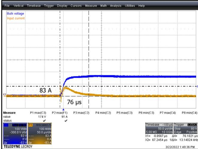
Figure 14. Inrush Current for  $V_{IN} = 115 \text{ VAC}$  and  $100 \mu\text{F}$  Input Capacitor with MinE-CAP IC Circuit.
